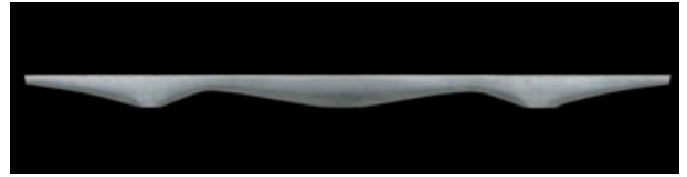
Figure 2.18: Concrete beam made with fabric formwork
